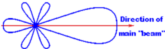
Fig 4. Radiation pattern of Yagi Uda antenna
