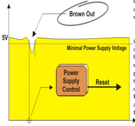
Brown out is a potentially dangerous state which occurs at the moment the microcontroller is being turned off or when power supply voltage drops to the lowest level due to electric noise.
