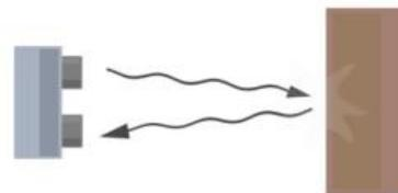
Basic Ultrasonic Sensor Operation
