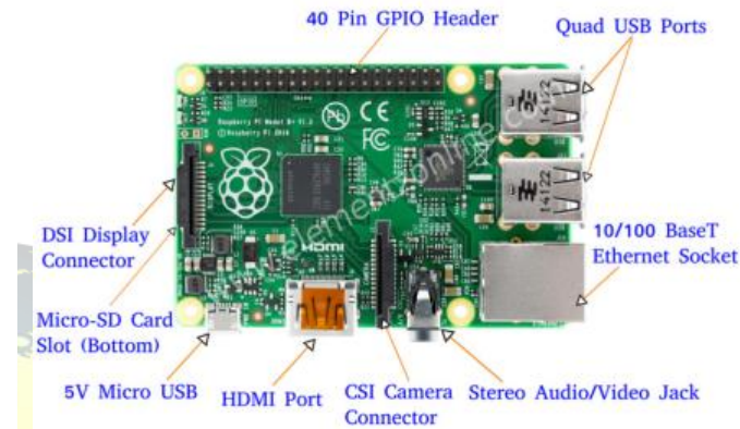
Figure 3 : RASPBERRY PI 2 and its features
