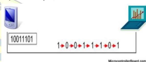
Transmitting the word 10011101 using serial communication.
