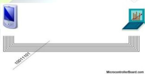
Transmitting the word 10011101 using parallel communication.
