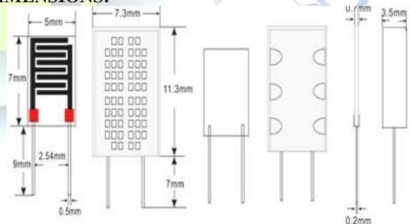
HR202L hygistor are the new moisture-sensitive components of organic polymer materials, has a sense of wet wide range, fast response, anti-pollution ability, without heating the cleaning and long-term use of reliable performances and many other features.
