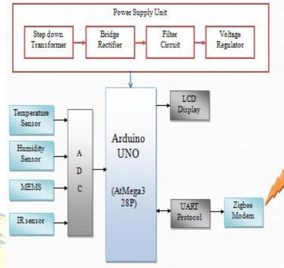
The input from the sensors and the supply power is given to the arduino UNO. UART protocol is used between the arduino and the zigbee module, which is a wireless mesh network.
