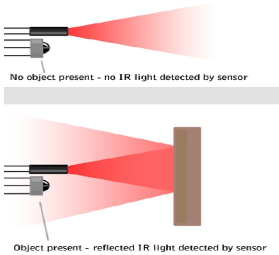
The specific light sensor to detect a select light wavelength in the Infra-Red (IR) spectrum up to the wavelength of 700nm -1mm and the frequency of about 300GHz to 430THz. Usually the IR light passes in a straight line. If any object is detected as disturbance near the track, then the rays will be reflect back and the alert message will be send to the control station. It has high reliability and radiant intensity.
