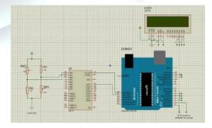
Weight of the canister is measured and converted to electrical signals using a load transducer and it is send to the programmable microcontroller. Using a Wi-Fi module, the information is passed to the mobile application. This application allows the user to set a
