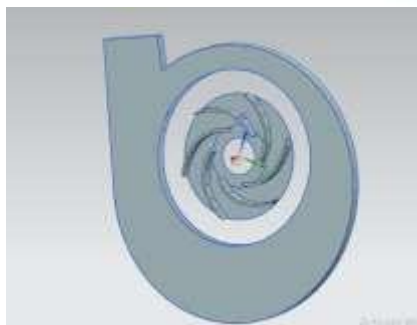
Fig. 6. Impeller and casing design for CFD analysis
