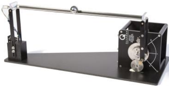
Fig 1: Quanser Ball and Beam System
