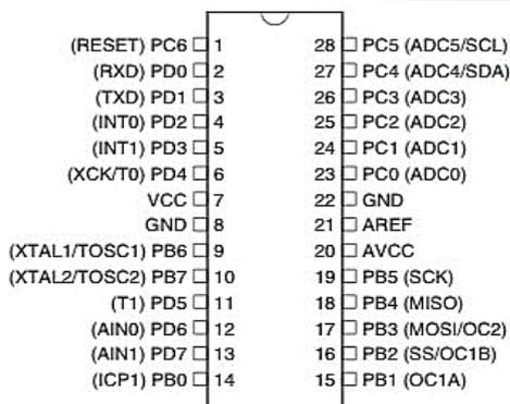
**Fig.3.3 Pin diagram of ATMEGA328**
