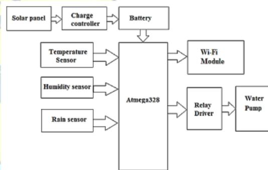
**Fig.3.1 Block Diagram of Wireless sensor unit (WSU)**
