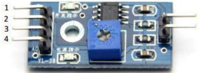
**Fig.3.16 Pin diagram of Rain Sensor Module**
