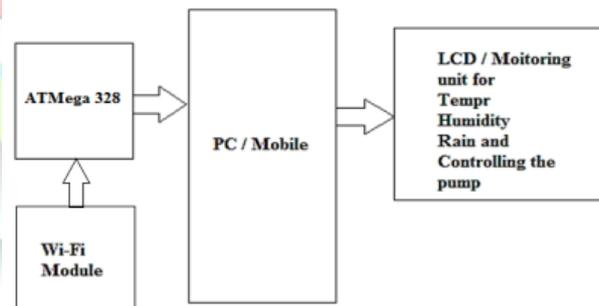
**Fig.3.2 Block Diagram of Wireless Information Unit (WIU)**
