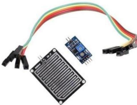
**Fig.3.15 Rain Sensor Module**
