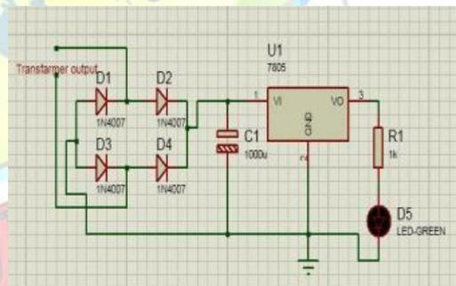
**Fig.3.17 Circuit diagram of power supply**
