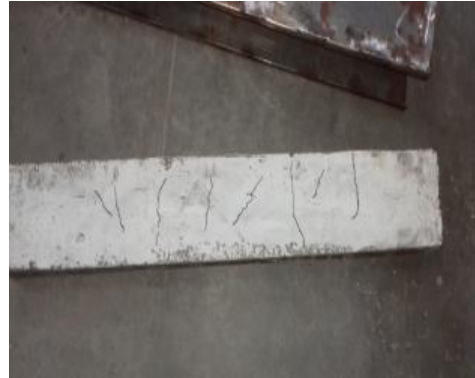
Fig 10 crack pattern in encased beam
