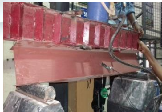
Fig 7 failure of back to back channel section
