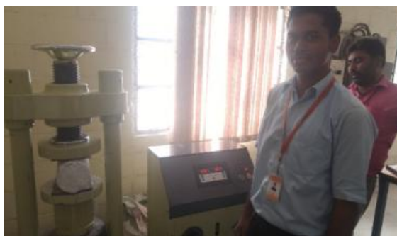
Fig 3.4 Split Tensile Strength Test (Cylinder 150mm dia and 300mm height)
