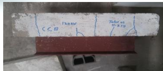
Fig 5.2 Crack pattern of conventional composite beam
