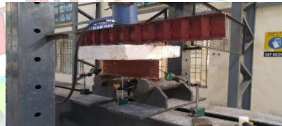
Fig 5.1 Shear connector welded composite beam
