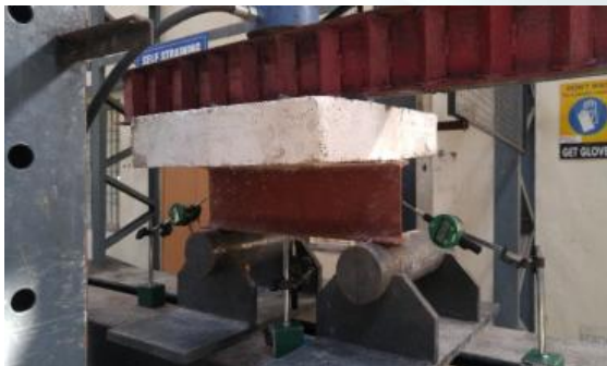
Fig 5.5 Shear connector welded Ferro cement self-compacted concrete composite beam
