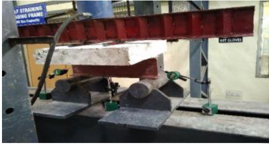
Fig 5.3 Shear connector welded Ferro cement composite beam
