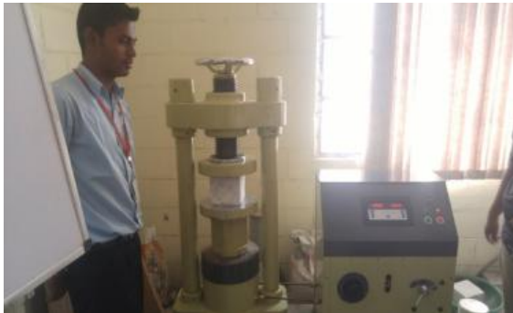
Fig 3.2 Compressive Strength Test (Cubes 150x150x150mm)
