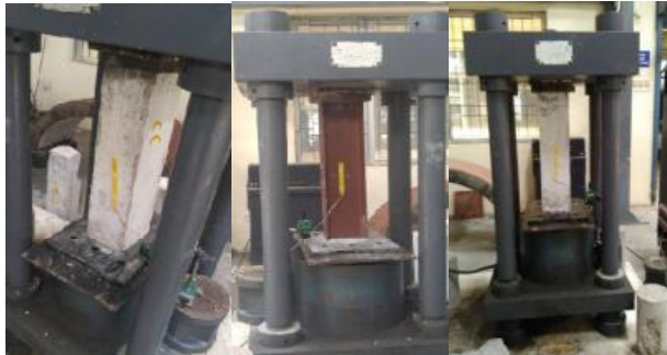
Fig 5.1 Test Specimens (a) Proposed Composite column, (b) Conventional RC Column, (c) Conventional Steel Column
