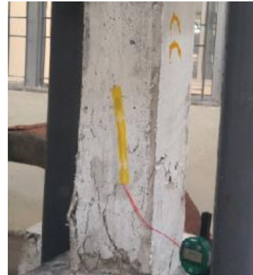
Fig 5.3 Failure pattern of Conventional RC Column
