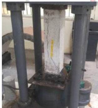
Fig 5.2 Failure pattern of Steel-Concrete Composite column
