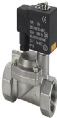
A solenoid valve is an electromechanically operated valve. The valve is controlled by an electric current through a solenoid: in the case of a two-port valve the flow is switched on or off; in the case of a three-port valve, the outflow is switched between the two outlet ports. Multiple solenoid valves can be placed together on a manifold.
