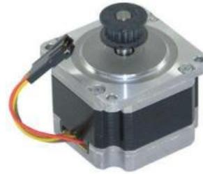
A stepper motor or step motor or stepping motor is a brushless DC electric motor that divides a full rotation into a number of equal steps. The motor's position can then be commanded to move and hold at one of these steps without any feedback sensor (an open-loop controller), as long as the motor is carefully sized to the application in respect to torque and speed.
