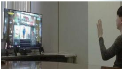
Fig. 1 Pointer type hand gesture interface on commercial smart TV.
