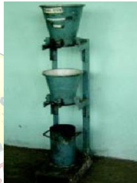
Figure 4.1.2 Compaction factor Apparatus
