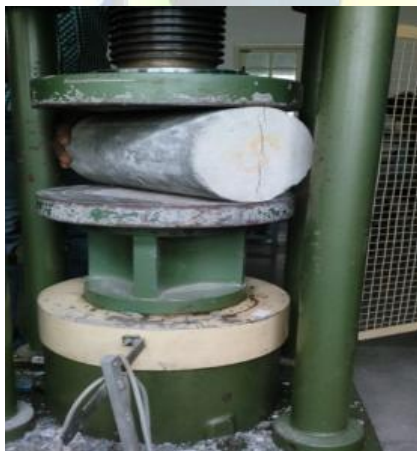
Figure 4.3: Split tensile Test
