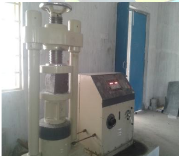
Figure 4.2: Compressive Strength Test
