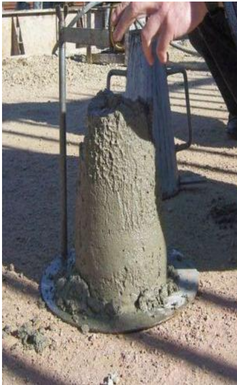
Figure 4.1.1 Slump height measurement
