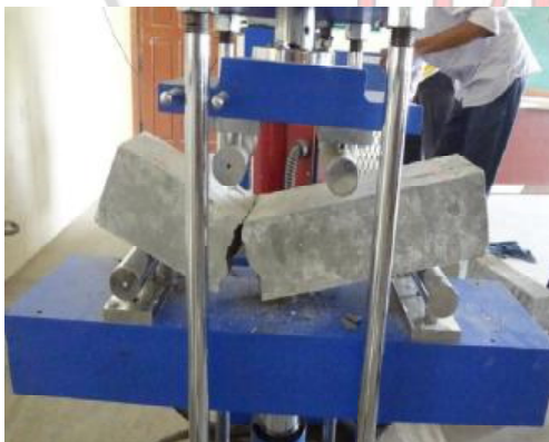
Figure 4.4. Flexural Strength test
