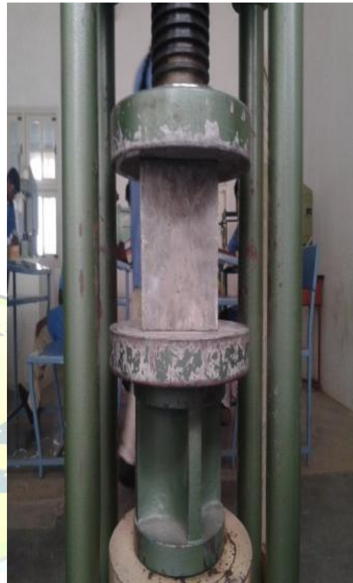
Figure 4.2: Compressive Strength Test
