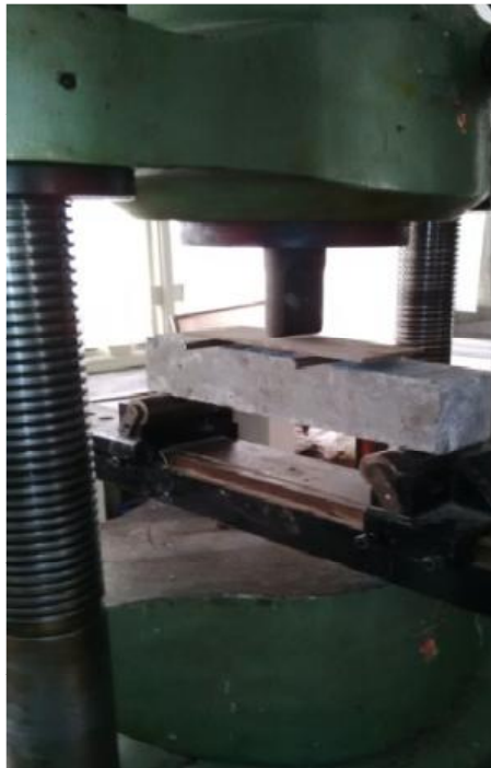
Figure 4.4. Flexural Strength test
