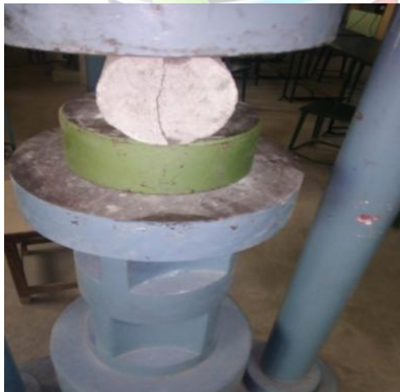
Figure 4.3: Split tensile Test
