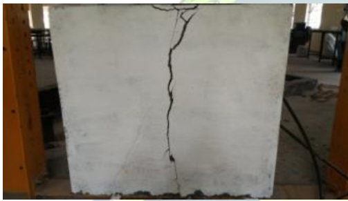
Figure 4.1 Failure Mode with conformed chicken mesh
