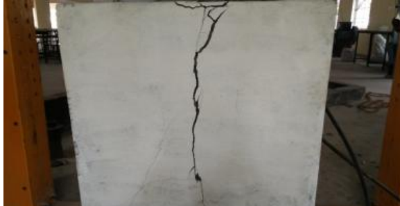
Figure 5.1 Failure Mode with conformed chicken mesh
