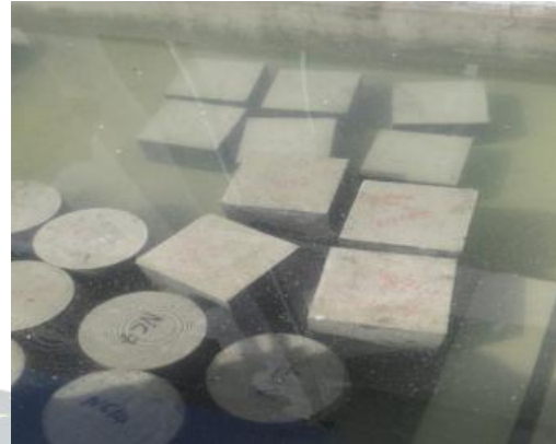
Figure 4cubes and cylinder of concrete replaced with fly ash and sea shells aggregate
