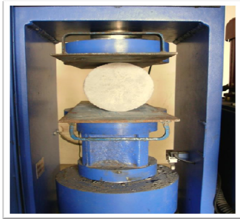
Figure 2 Tensile testing of cylinder
