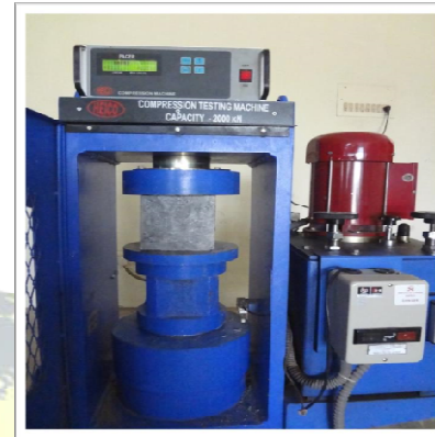
Figure 1 Compression Testing of Cubes
