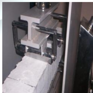
Fig 8: Flexural strength Test
