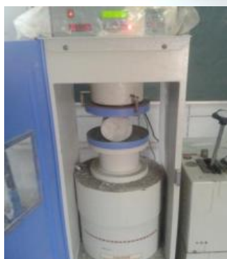
Fig 9: Split Tensile Test
