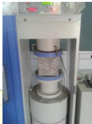
Fig 9. Compressive strength Test
