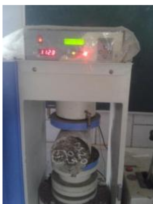
Fig 10. Split Tensile Strength Test
