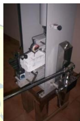
Fig 11. Flexural Strength Test
