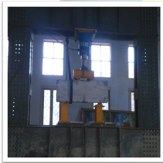
Fig 7 Flexure Test on Beam
