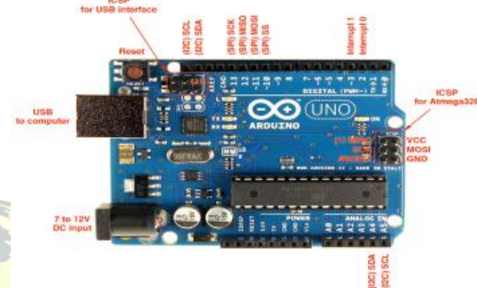
Fig 3.2:Arduino board with pin details
