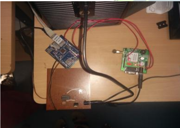
Fig 5.2:Amplifier circuit connected with Arduino interfaced with network module and connected to GSM
