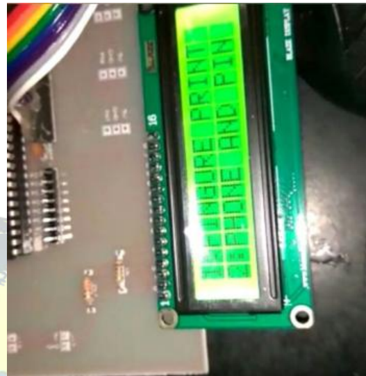
Figure 3, LCD module displaying the request for finger print or personal identification number
