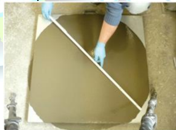
Figure 5: M170 with 0.99 vol.-% steel fibers
