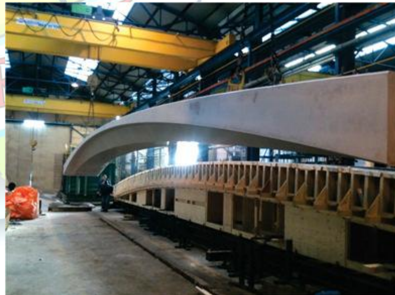
Figure 1: Goosebridge, fiber-reinforced UHPC, no steel bar reinforcement inside; production: Romein Beton, NL; material development: G.tecz Engineering, Germany Ultra High Performance Concrete – Sustainable and Cost-effective
