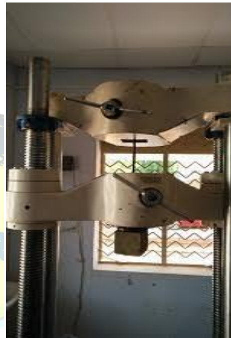
Fig. 4.1. Pull out test in UTM
