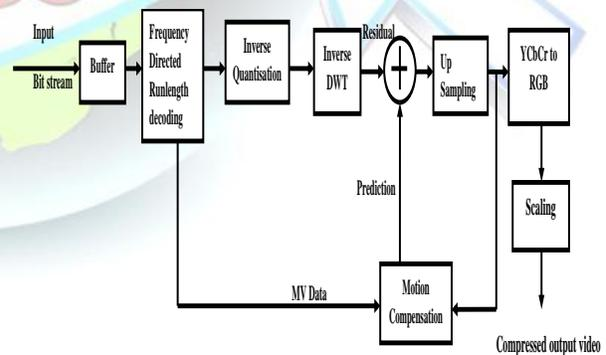
Figure 2 Block Diagram of Decoder
