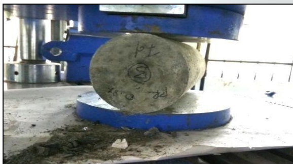
Fig.3 Split tensile test of cylinder
