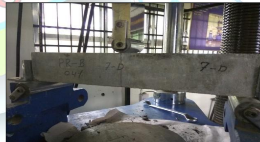
Fig.5 Flexural strength test of beam
