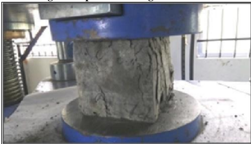
Fig.2 Cube failed under the Load
