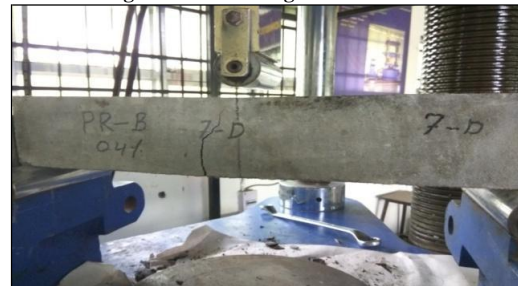
Fig.6 Beam failed under the load
