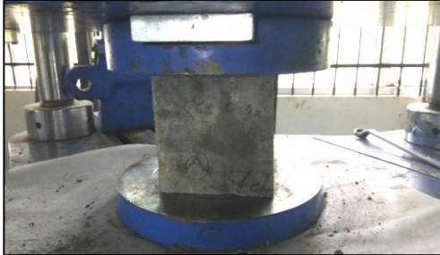
Fig.1 Compressive strength test of cube
