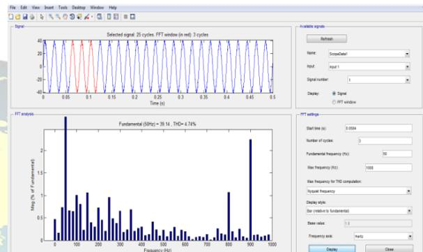
Fig. 3 Output of Total Harmonic Distortion after Filtering
