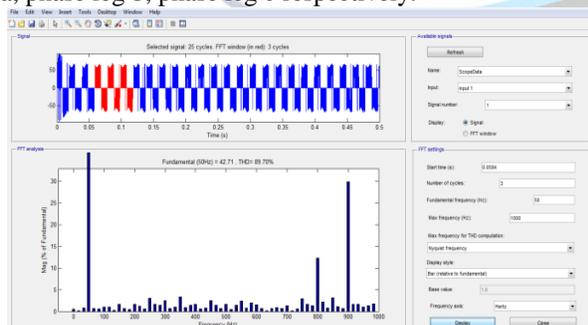
Fig. 2 Output of Total Harmonic Distortion before Filtering
