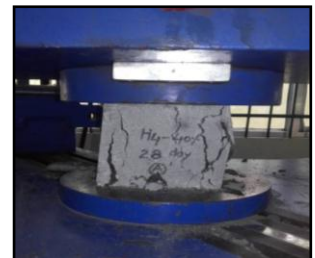
Fig.4. Compression Test
