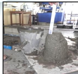
Fig.3. Slump Test
