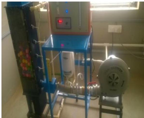
Fig 1. Schematic diagram of fluidized bed cooling tower
