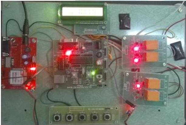
The project output data's are send to android application and all the modules are controlled by smart phone.
