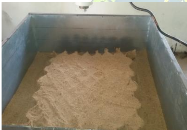
Figure 4: Coir geocell mattress filled with sand
