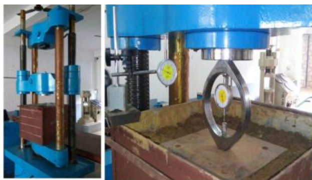
Figure 4: Load Setup and Apparatus
