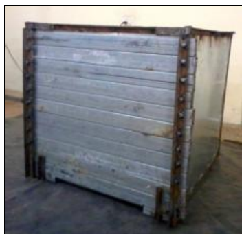
Fig. 1 Test tank fabricated for the model study
