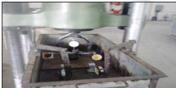
Fig. 3 Test setup for shear loading
