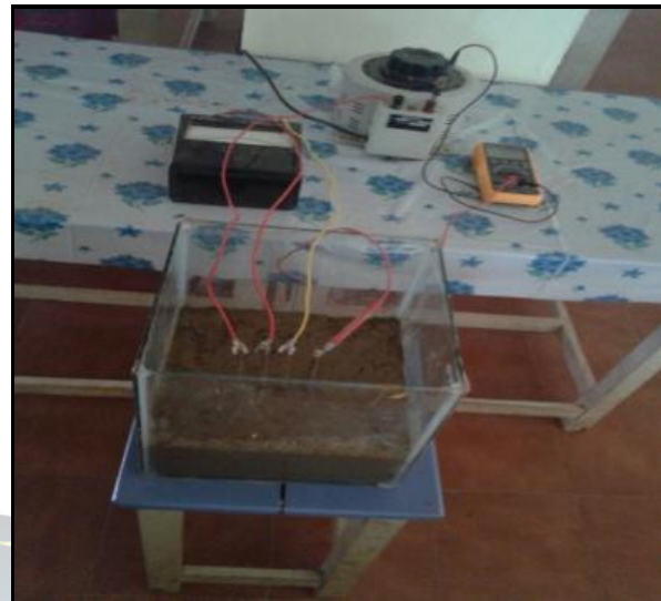
Fig. 2 Test setup –wenner array
