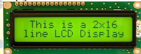
We have used 2\*16 LCD (Liquid Crystal Display), consisting of 2 rows & can display 16 bits in a row, to display our output for our Convenience. We also have used the Preset to adjust the contrast & brightness of Liquid Crystal Display.
