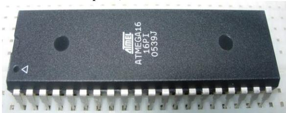
It requires only 131 instructions which are mostly executed by a single clock cycle of frequency 16MHz. Piezo Electric Crystal of frequency value 3.86 MHz is used to give a clock cycle frequency to the Microcontroller. It consists of 32 pins divided into 4 ports A, B, C, D, each port consisting of 8 pins which perform dual functions.
