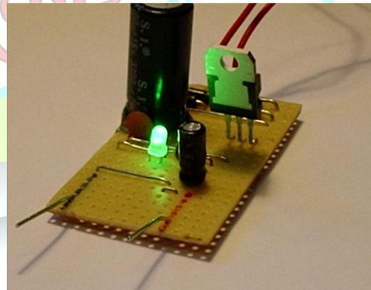
We also have used LED (Light Emitting Diode) to indicate that the Power Supply is on. We have used a dropping Resistor which acts as a Voltage Limiter to supply a voltage value of 2V to LED & the remaining 3V is dropped across the resistor. Thus we have a Regulated Power Supply of 5V to our Project.
