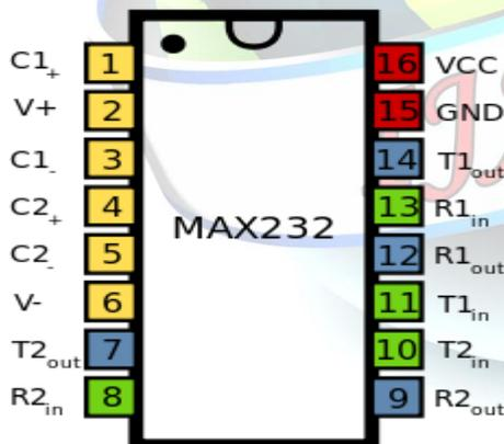
The Level Converter acts as a Voltage Interpreter between Laptop & Microcontroller .We have used Four Capacitors which acts as Voltage Double.
