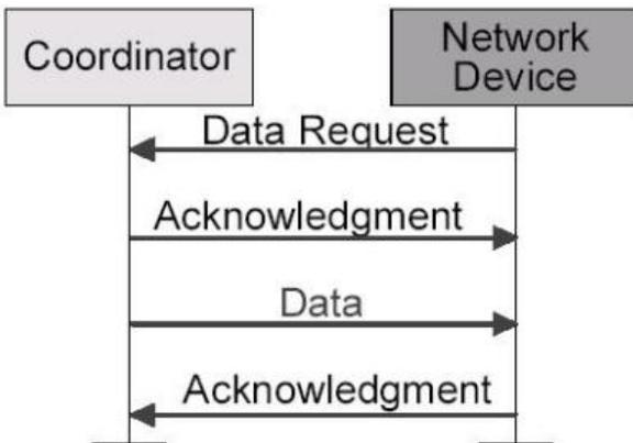
Fig ii) Communication from a coordinator in a non-beacon-enabled network
