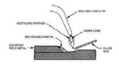
Fig.1 Fusion welding
