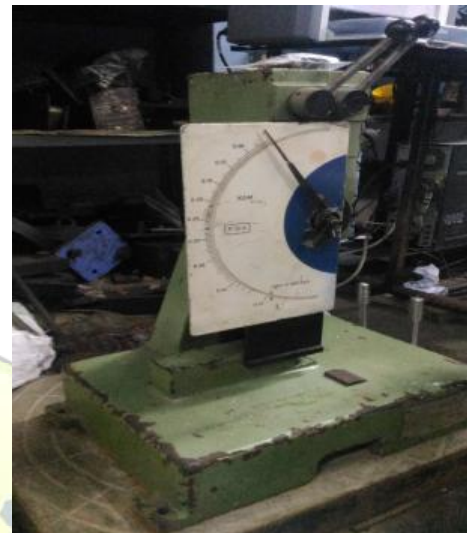
Figure-4-Izod impact testing machine
