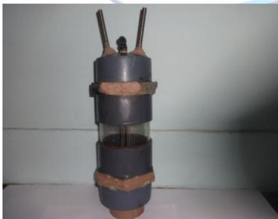
Fig. 1 hydroxy generator
