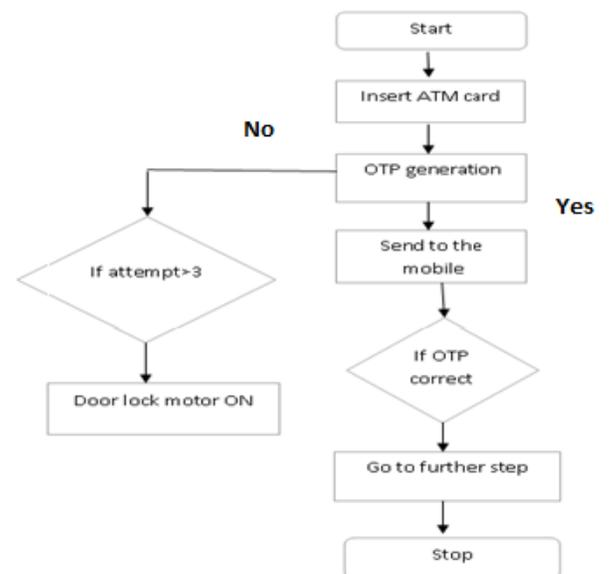
If theft occurs in the ATM machine, information is sent to the respective banks. In proposed system we implement one-time password generation (OTP). Every time user the inserts the card, one-time password will be send to the respective card holder's mobile number. The user can access the ATM card only by entering the correct OTP.
