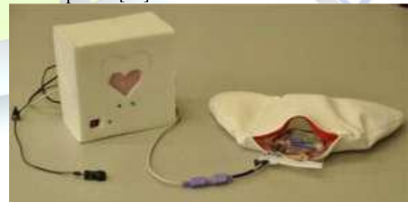
Fig. 1. Prototype with the Mimo recorder (left) and the smart pillow (right).
