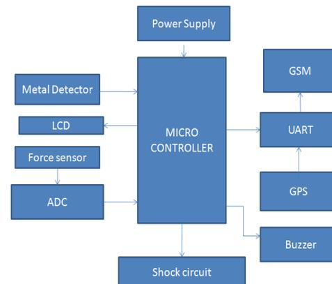
When a force which is higher than the threshold value is applied to the women, it was detected by the force sensor and system incorporates a screaming alarm that uses a buzzer to call out for help. Since the force sensor output is analog, it is given to the ADC to get the digital output.
