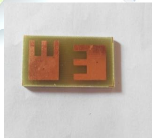
Figure. 8 photograph of fabricated antenna
