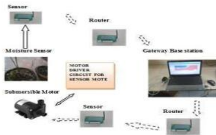
Fig.2. Block Diagram of Proposed Smart Irrigation System
