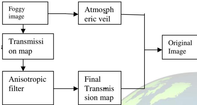
In the proposed algorithm, the foggy images from the camera is given as an input and the scene depth of the image is calculated and the transmission map of the foggy image is calculated and then the output of the mapped image is given as an input to the anisotropic filter.
