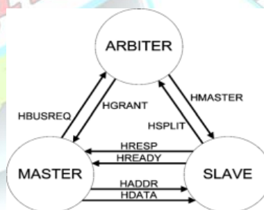
Fig 1 AHB Based Connection among Bus Arbiter, Master and Slave for Bus Split Operation
